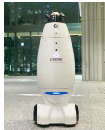
The autonomous moving security robot SQ-2 uses proprietary 3D laser sensors.
