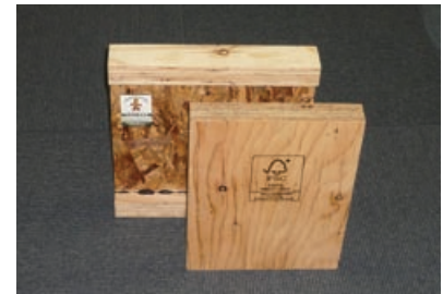
Japan-grown I-joist and LVL newly adopted
